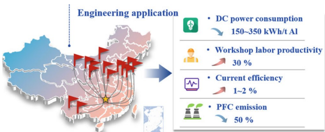
Figure 5. Result of Digital Twin implementation in Chinese smelters [18].
